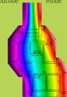
The cross section above shows how the multi-chambered profile prevents the transfer of heat from the inside to the outside.
